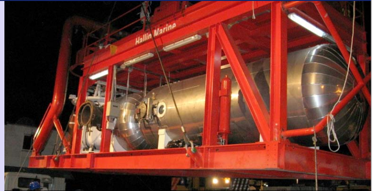
The living area being prepared for delivery: it can house 12 divers for up to a month
